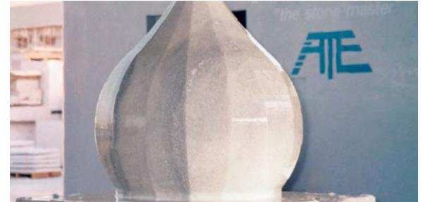
Data input for the profile to be cut is simple, even for personnel without computer knowledge, thanks to our exclusive program. The linear speed of the diamond wire can be adjusted from 0 to 40 m/sec, depending on the type of stone, under the control of an inverter. The cutting speed varies from the set maximum based on the complexity of the cut. Wire tensioning is hydraulic.
